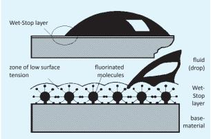
The fluorinated molecules of the high-purity Wet-Stop layer adhere very strong on the surface. The Wet-Stop coating acts as a network whose fluorine "bristles" repel the fluid.
