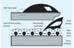
The fluorinated molecules of the high-purity Wet-Stop layer adhere very strong on the surface. The Wet-Stop coating acts as a network whose fluorine "bristles" repel the fluid.
